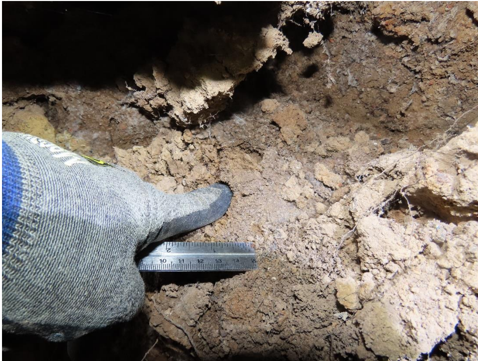
Photo 15: The soil yielded to finger pressure.
